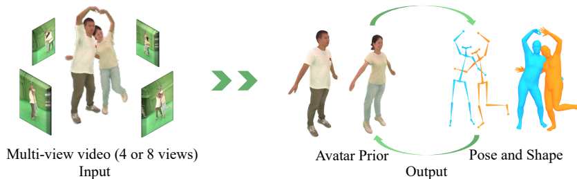
Fig. 1: We propose AvatarPose, a method for estimating the 3D poses and shapes of multiple closely interacting people from multi-view videos. To this end, we first reconstruct the avatar of each individual and leverage the learned personalized avatars as priors to refine poses via color and silhouette rendering loss. We alternate between avatar refinement and pose optimization to obtain the final pose estimation.
